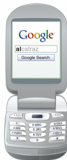
Figure 1: An example query prediction interface used with Google mobile search: The user has typed in the letters “al”, and after considering her location (that she is in San Francisco, CA) we suggest the most probable completion of the prefix: “alcatraz” (shown in faded grey)
